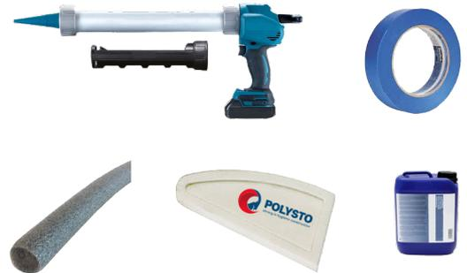
When the joint width exceeds 6 mm, place a foam backing rod in the joint 3 mm deeper than the surface of the kerb. This is to prevent overuse of HygiSeal and to speed up the curing time of the joint.
